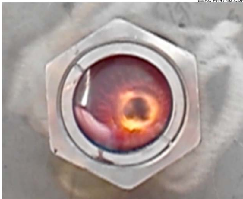
Figure 5. Image of the stable flame in the microturbine operating on 100% syngas.
